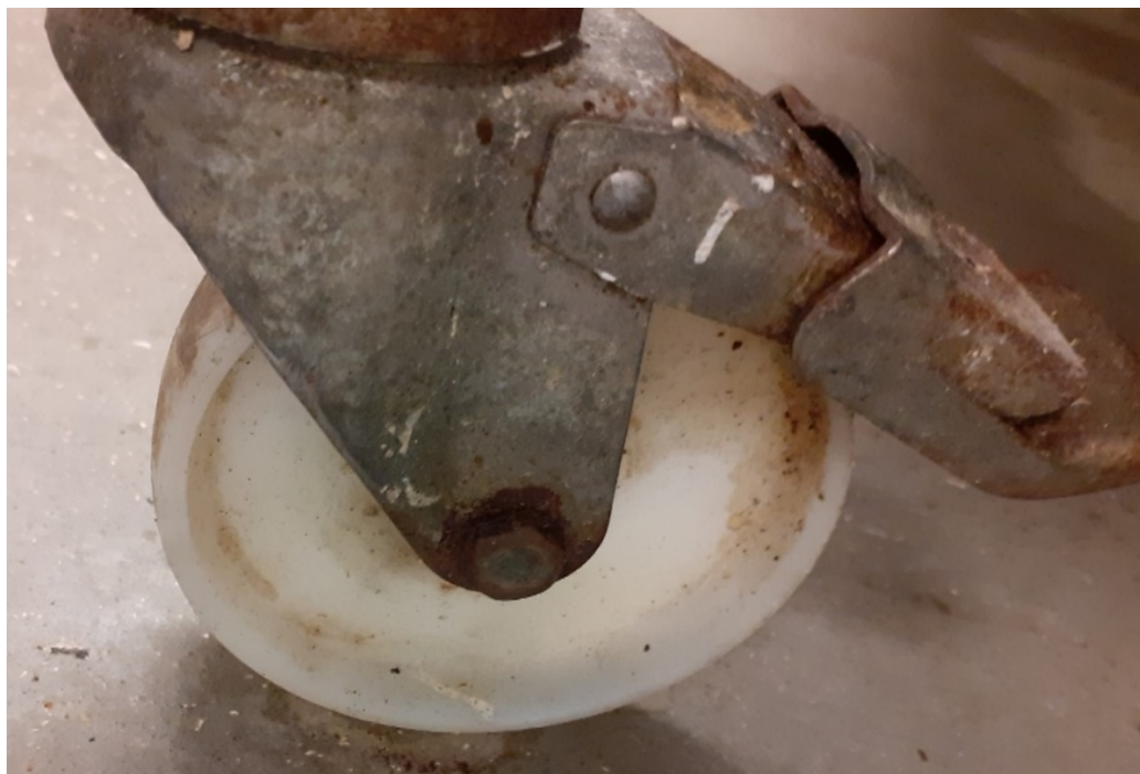
Figure 7 Shows a trolley wheel, the trolley is adjacent to the dish wash area. The wheel and housing are dirty, and the housing is rusting and no longer able to be kept clean.
