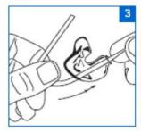
Pull the tube until the bend reaches the mould. All the tapered section should have come through the other side.
