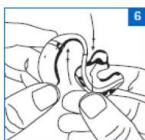
Push the end of the tubing onto the plastic nozzle on your hearing aid.
