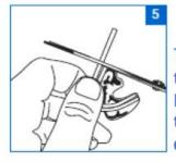
Take the old piece of tubing you saved and line it up with the newly threaded tube. Cut the end to the same length.
