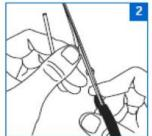
Cut the last 5cm (2 inches) of a pre-bent piece of tubing to a tapered end.
